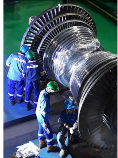
The detailed inspection revealed some of the erosion shields would need to be replaced.
