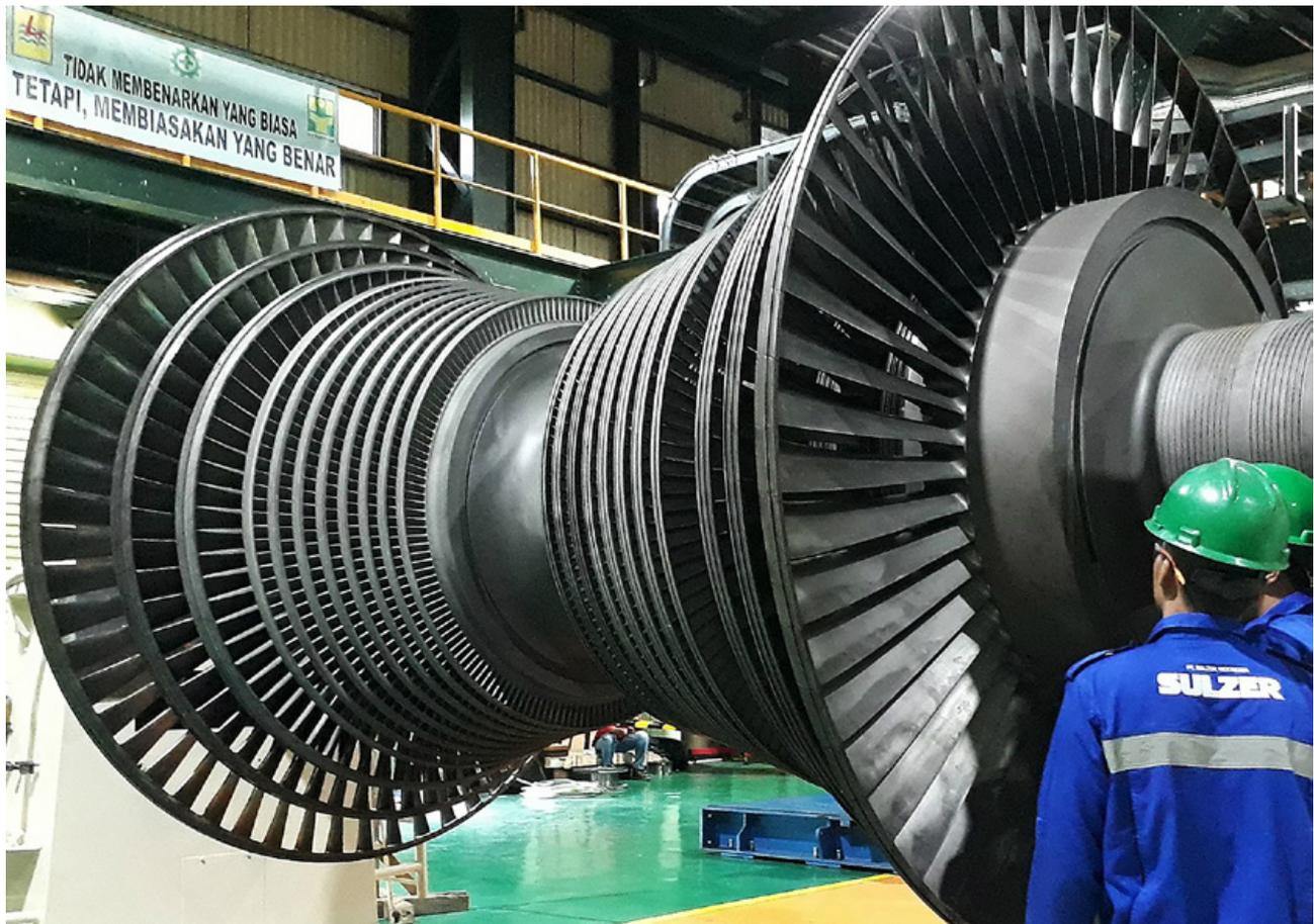
The turbine rotor was also balanced before being reassembled.
