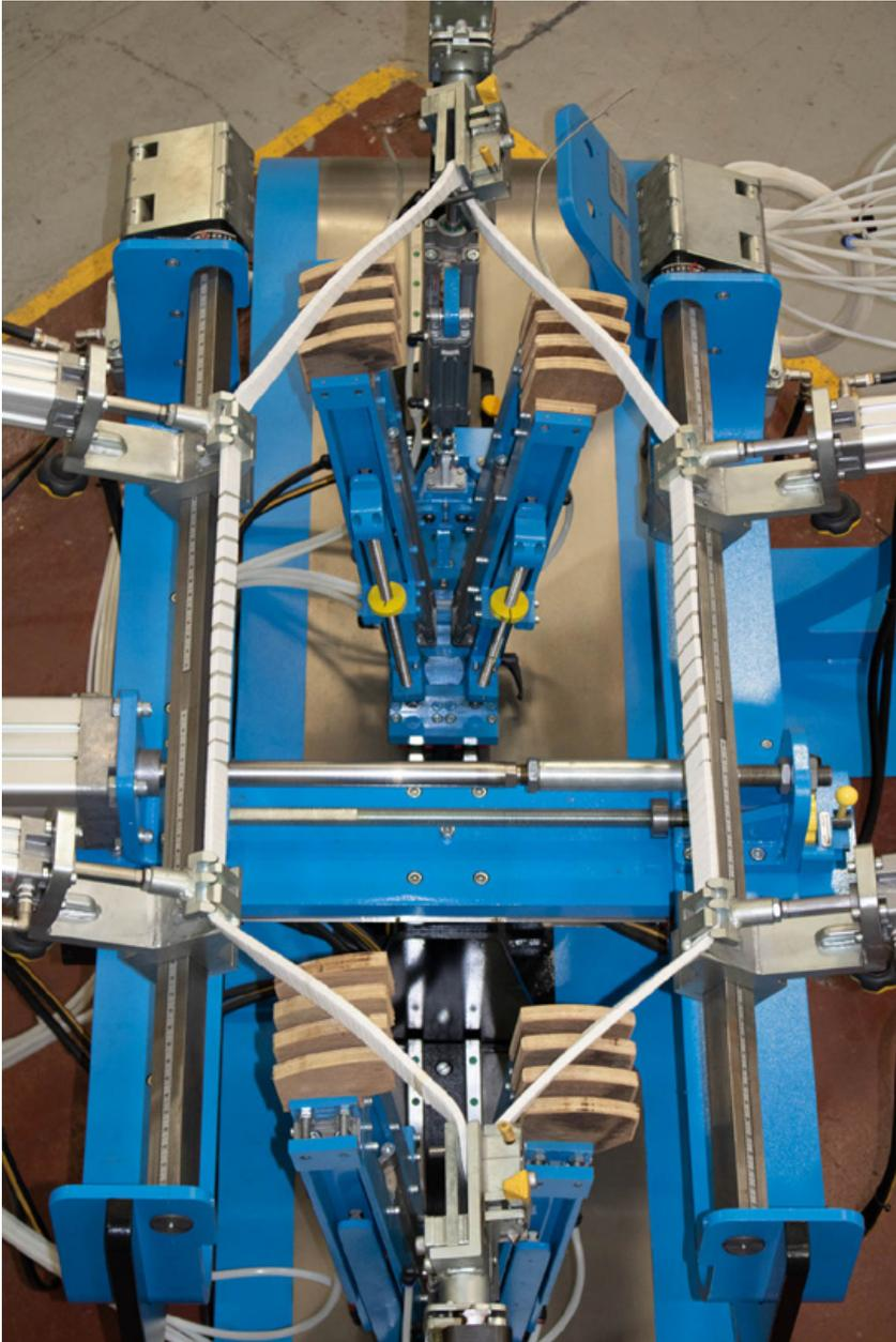
***"While traditionally only a few select workers would be entrusted to apply the radii to a coil, the Radius Forming Coil Spreader allows the task to be completed accurately with high repeatability – minimising hammering post processing."***
