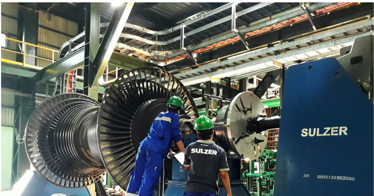
Preparing the turbine rotor for balancing
