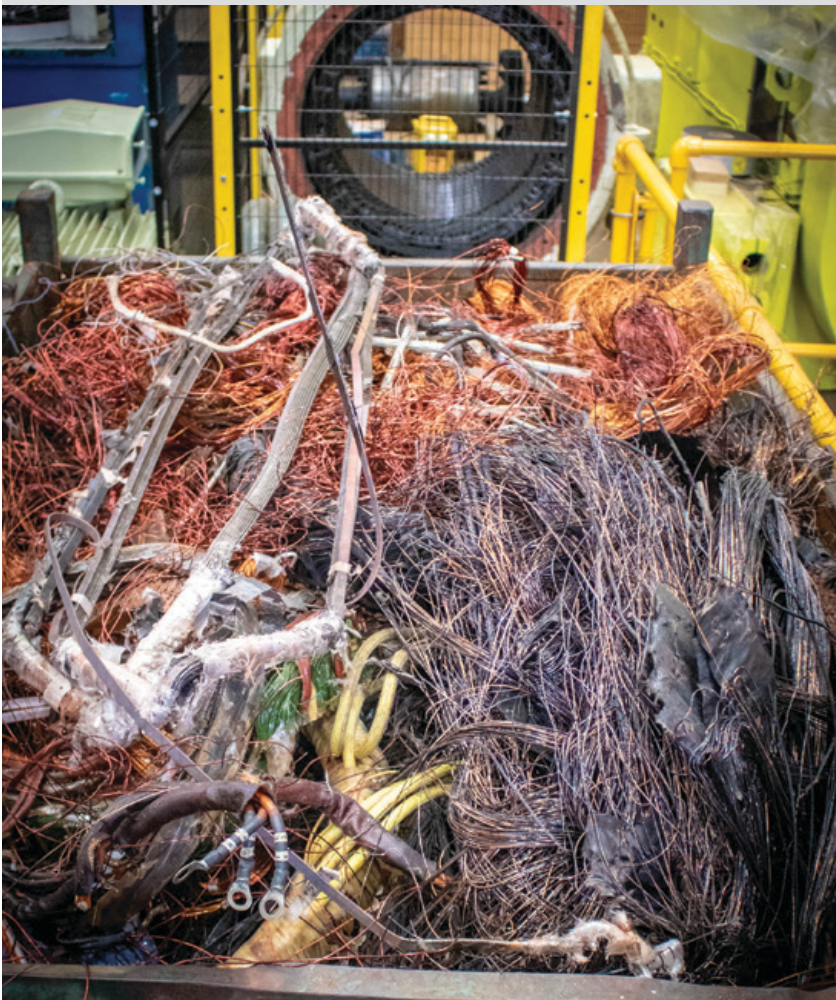
To commit to a sustainable future, everything that can be recycled is stripped from the motor, including the oils and greases in water butts and the copper stripped from within the motor.
