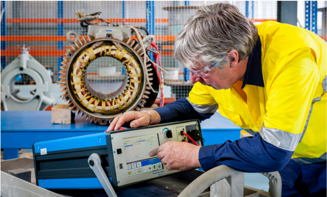
Electrical testing after rewind - credit Sulzer.
