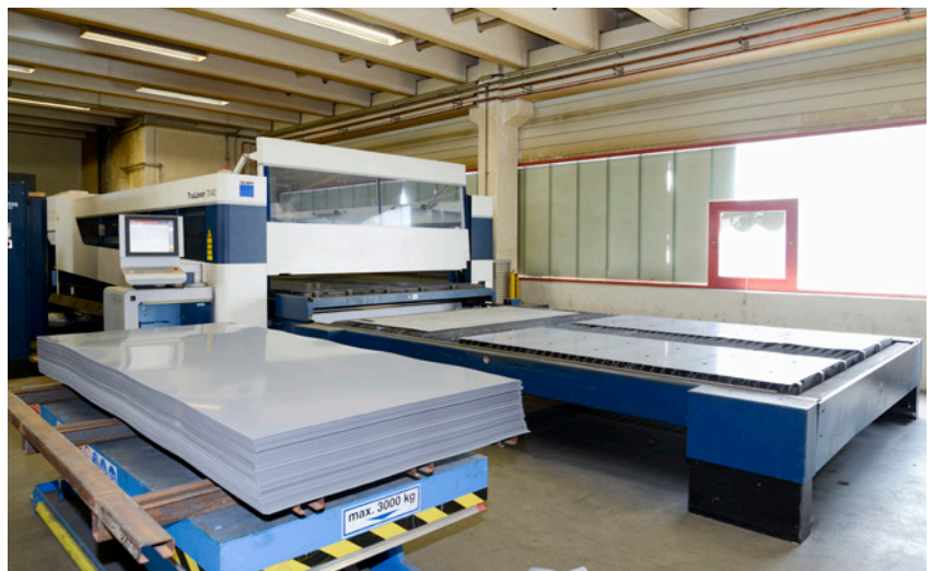
The free programmable machine control of the double head-laser cutting units allows the production of any desired contour for the electric machine.
