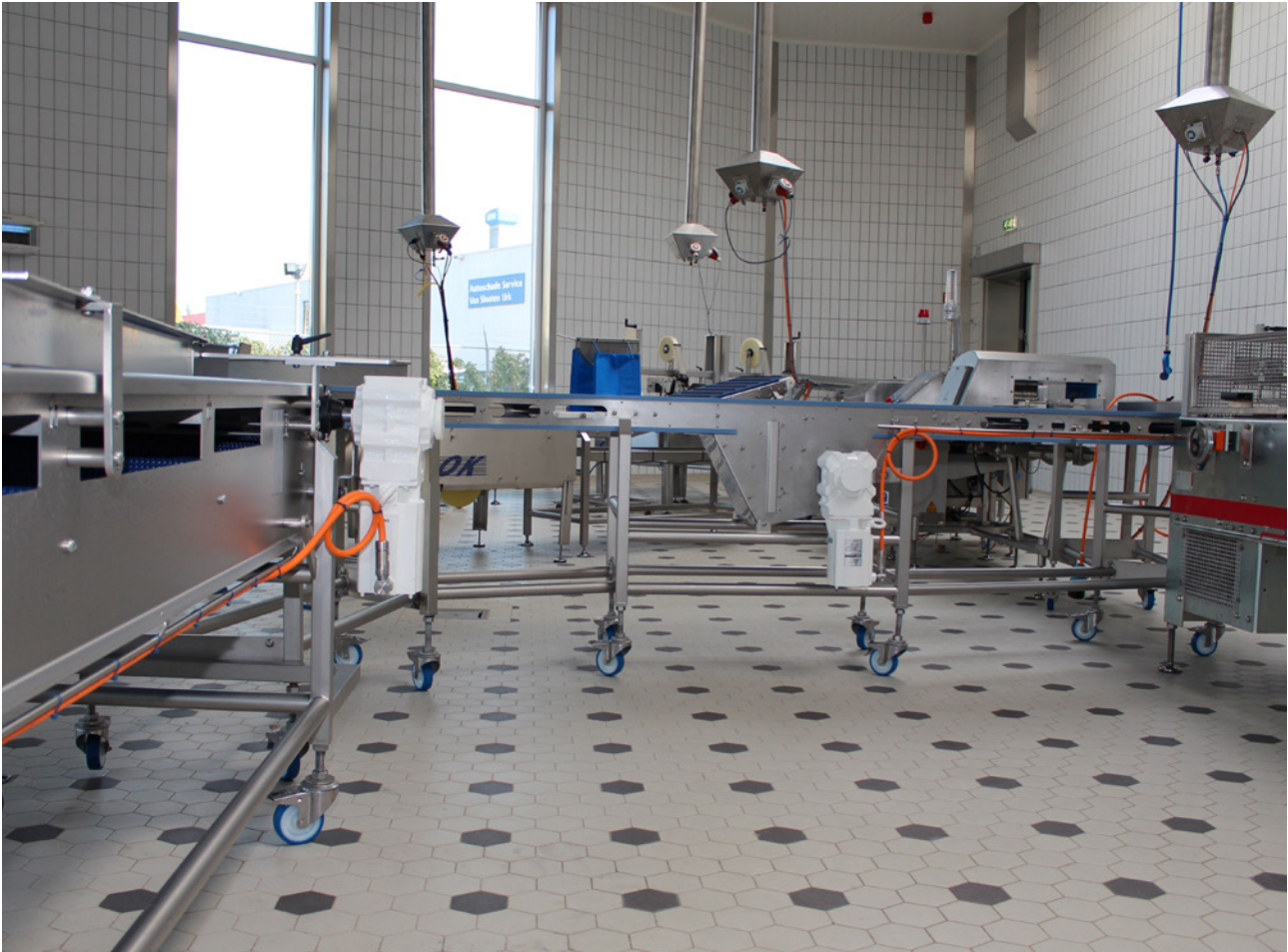
The fish processing lines can be reconfigured for different products
