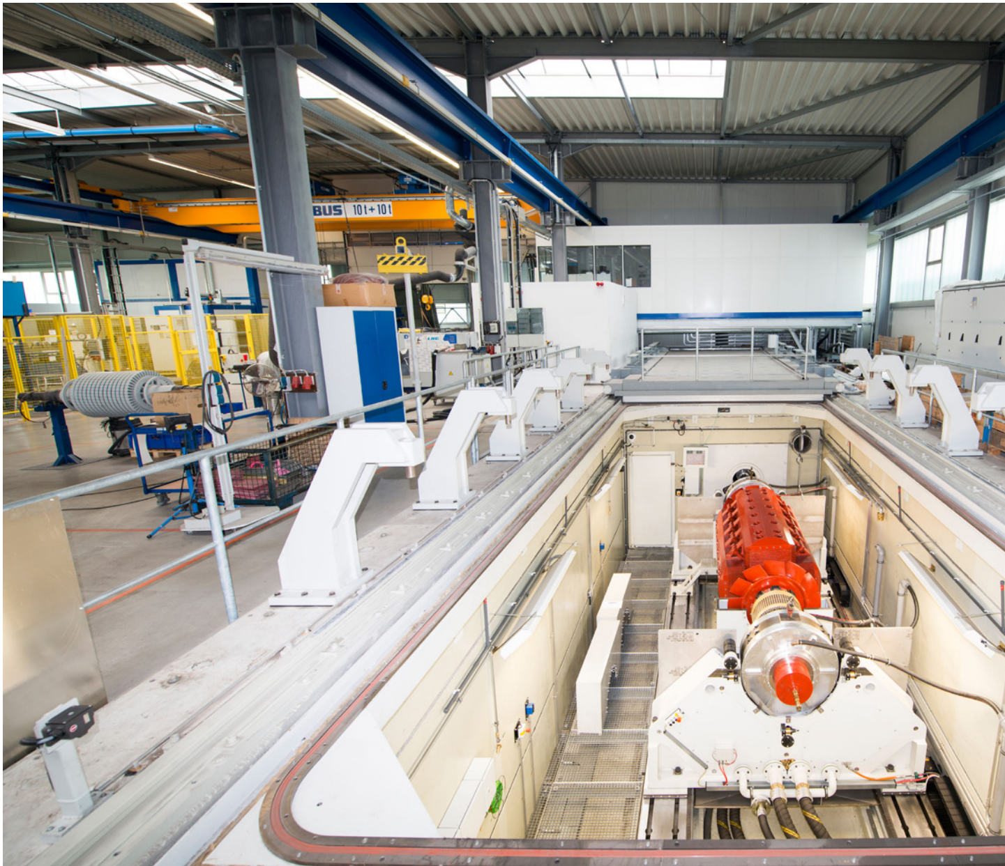
High-speed balancing service for rotors up to 32 tonnes.
