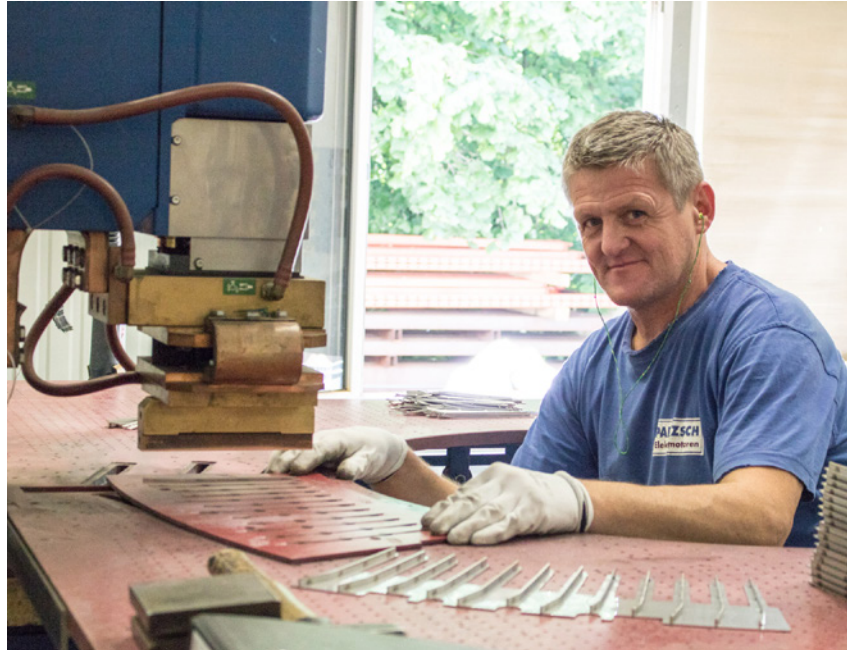
Spot welding air gap spacers onto stator laminations is an automated process, and an option offered by PARTZSCH.
