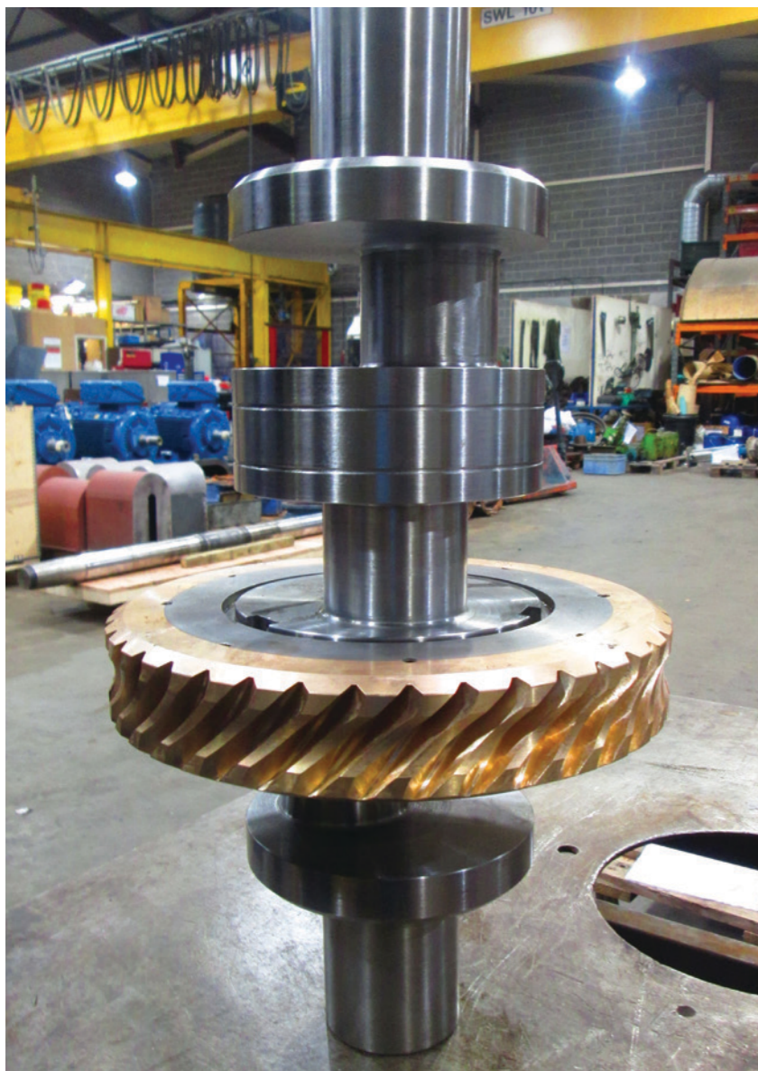
Fig 3. A new pinwheel and worm had to be made.
